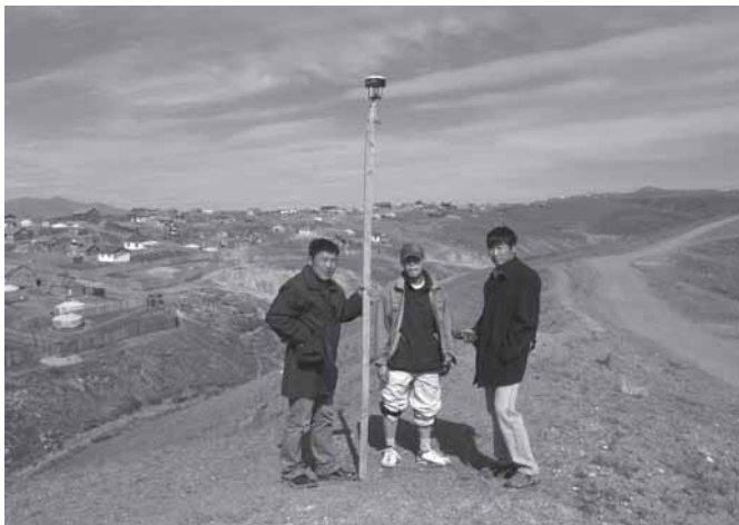
The area surrounding the Lama's excavations and our test excavations were surveyed using high precision GPS equipment. Erdene Batshatar, Tsend Amgalantugs, and Enkhtur Altangerel are using the Ashtech/Magellan Rover unit to record longitude, latitude and elevation of selected positions. Data is later downloaded to a small computer and the results can be observed and used shortly afterwards.
